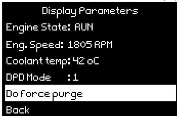
The relevant data parameters will be displayed, including coolant temperature and DPD Mode. The purge will start when conditions are correct, including coolant temperature at 158°F. The timer will count up to 780,000ms. Purge complete. If the purge will not initiate or will not complete, the engine may require additional diagnostics or service.
